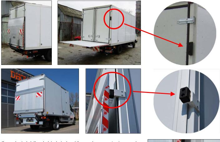
• If a mechanical platform lock is desired, and the rear doors cannot swing around a fixed locking plate mounted to the rear frame of the body, pivoting locking plates are available in different lengths from DHOLLANDIA spare parts department.
