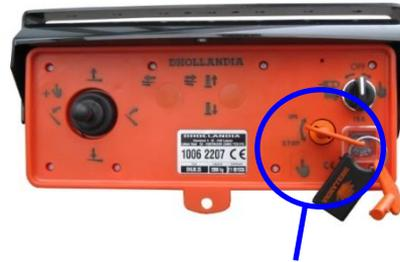
Turn clockwise to switch battery power ON
