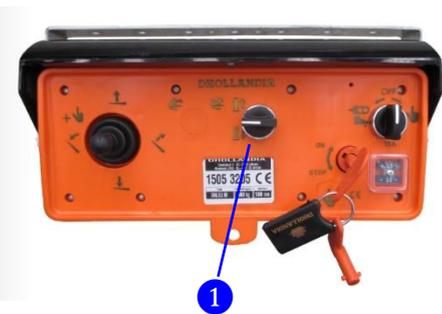
When the tail lift is equipped with hydraulic stabilising legs, the control units above are completed by a turn switch to push the legs down or pull them up.
