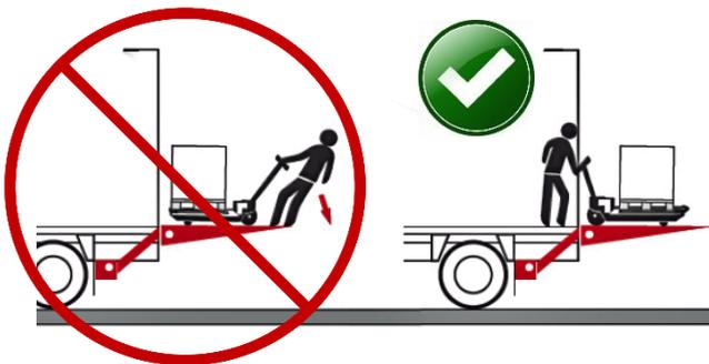
NEVER pull the load from the vehicle onto the platform. ALWAYS push it out. Pulling the load from the vehicle can result in a fall from the platform and cause serious injury or death.
