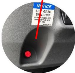
Push button to switch tail lift power ON (indicator light on)
