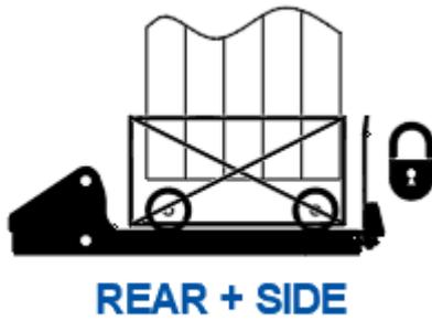
Before lifting or lowering loads, make sure the loads are secured on the platform surface. Deploy the hinged ramps or roll stops (if so equipped), lower loads on a pallet jack down on the platform, surface or immobilize the load via equivalent securement device.
