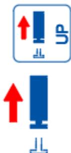
If so equipped, raise the mechanical or hydraulic stabilizing legs into travel position.
