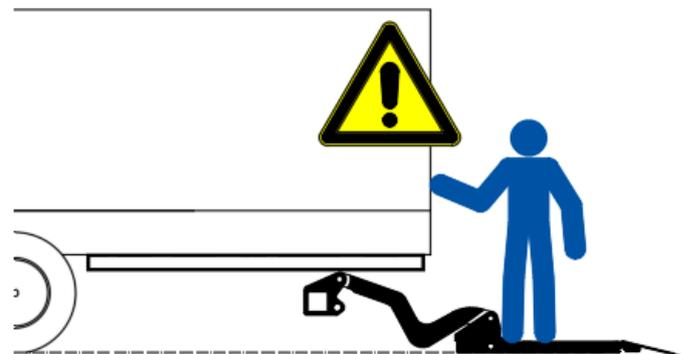
When riding on the platform, make sure you stand min. 25 cm away from the inboard platform edge, make sure your footing is solid, and ALWAYS maintain 3 points of contact. [see 7.4 on page 24]
