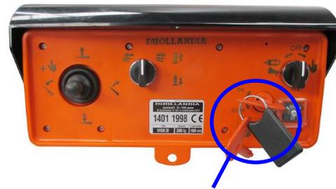
Turn clockwise to switch battery power ON
