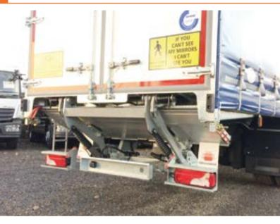
The DH-RM.20 is an extremely versatile and robust lift, equipped with a wide arm center and 2 lift cylinders. It offers a level ride between the vehicle floor and the ground, plus automatic tilt at ground level. This premium lift is the best suited fold-away lift for demanding distribution, incl. high stack pallets and roll cages.
