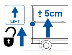
LIFT the platform approx. 5 cm to take the platform weight off the stow lock or pins.
