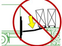
NEVER use a foldable platform as a bridge plate between the vehicle floor and a loading dock. Keep the platform securely stowed in its travel position to avoid damage.
