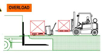
Whenever cargo is loaded or offloaded with forklifts, electric pallet jacks, and the total weight of the load plus handling equipment exceeds the maximum rated capacity of the tail lift, ALWAYS use a dock plate from the loading dock to the vehicle floor, and safely stow the lift below the vehicle floor level, or in the pocket or brief case under the loading dock.
