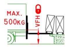
Unless the vehicle suspension can be blocked (e.g. by means of hydraulic stabilising legs) and the floor maintained at the original height vfh, the max. load transferred over the platform should not exceed 500 kg. Exception: column lifts with 2 tilt cylinders [option OVH011].
