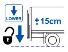
LOWER the platform approx. 15 cm to disengage the stow locks.
