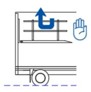
If applicable (e.g. on curtain-sider vehicle), deploy the guard rails, and lock them in vertical position.
