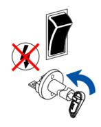
Switch off the electrical power to the tail lift (cabin switch or main battery disconnect switch in the external control box, or both if both are available). Close the cover of the control box.
