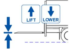
LIFT or LOWER the platform to the correct height for closing it. Normally approx. 15 cm below the vehicle floor.
