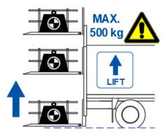
LIFT the platform off the ground, with respect for the load charts. Above roof level, limit the load to 500 kg max. ALWAYS release the button when you hear the hydraulic system go in overpressure.
