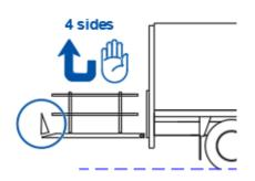
Unless unfolding automatically, deploy ALL guard rails and lock them in vertical position.
