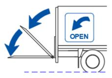
OPEN the platform into horizontal work position.
