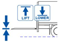
LIFT or LOWER the platform to the correct height for closing it. Normally approx. 15 cm below the vehicle floor. Use the HEIGHT DETECTION TO CLOSE for your convenience.
