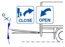
Adjust the platform pitch to compensate for the slope of the ground [see §9.1 on page 46].
