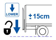
LOWER the platform approx. 15 cm to disengage the stow locks.
