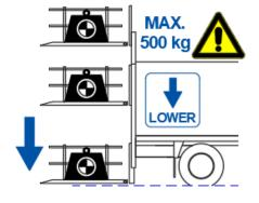
LOWER the platform to the ground, with respect for the load charts. Above roof level, limit the load to 500 kg max.
