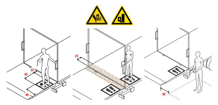
On the platform, from a safe operator position of minimum 40 x 40 cm square, clearly and permanently marked at minimum 25 cm distance from the hazard zone between the platform and the rear of the vehicle floor. Maintain 3 points of contact (see above).
