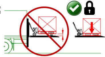
NEVER drop any load on the platform (ex. by means of a forklift, gantry crane, etc...). The impact of dropping a load is far greater than the nominal weight of the load and can cause severe damage to the tail lift.
