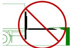
NEVER use a dock plate on top of a floating platform as a bridge between the loading dock and vehicle floor.
