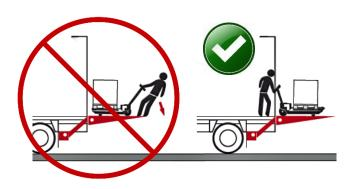
When using a second external lift to load or unload to the vehicle ground, NEVER pull the load from the vehicle onto the platform. ALWAYS push it out. Pulling the load from the vehicle can result in a fall from the platform and cause serious injury or death.
