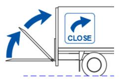
CLOSE the platform. Continue to press CLOSE until you hear the hydraulic system go in overpressure. Then release the controls.
