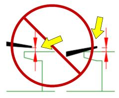
If the loading floor of the vehicle lowers or rises relative to the loading dock, use the electrical controls to adjust the platform position flush with the loading dock surface.
