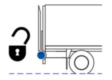
Observe all safety instructions and disengage the locking pins under the lift runners (if applicable).
