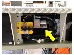
Safety valve on lift cylinder (DH-VO)
