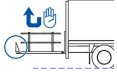
Unless unfolding automatically, deploy the guard rails and lock them in vertical position.
