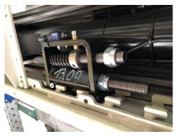
Calbe rupture detection inside cylinder beam (DH-VO)
