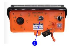
When the tail lift is equipped with hydraulic stabilizing legs, the control units above are completed by a turn switch to push the legs down or pull them up.
