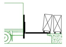
The tail lift can only be used as a loading platform if the dock is lower than the vehicle floor.
