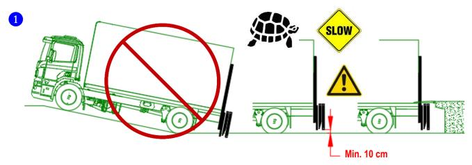
When the intention is to dock with the platform lowered below the vehicle floor level, DO NOT lower the platform until the vehicle is standing on flat even ground. ALWAYS revers slowly, and make sure you maintain sufficient ground clearance between the lowest part of the tail lift and the ground. Take into account variations in the suspension and vehicle height.
