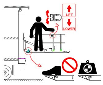
Similarly, if the platform is equipped with a hydraulic rentention ramp [ref. OVP152], that ramp is raised and lowered by a toggle switch [ref. OAE015.0]
