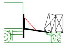
The tail lift can be used as a bridge plate, if it is equipped with the optional tilt cylinders with adjustable platform orientation [OVH011].
