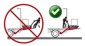
NEVER pull the load from the vehicle onto the platform. ALWAYS push it out. Pulling the load from the vehicle can result in a fall from the platform and cause serious injury or death.
