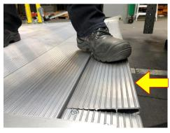
Standard toe-guard flap on exterior platform (DH-VO)
