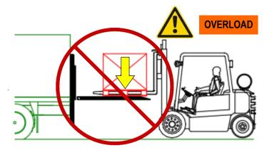
NEVER drive a forklift onto the platform. Driving a forklift onto the platform can cause severe structural damage, potentially
