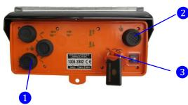
Push and hold to activate push buttons of main external control box Release to enable auxiliary control
