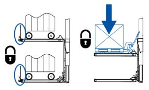
Before lifting or lowering loads, make sure the loads are secured on the platform surface. Deploy the platform cart stops (if so equipped), lower loads on a pallet jack down on the platform surface or immobilize the load via equivalent securement device.
