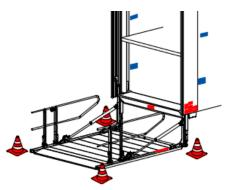
Decals [standard]. The tail lifts are supplied with a number of operation decals, load diagrams and safety decals, most of them to be applied to the vehicle body during installation. These decals must be kept clean and legible at all times, and replaced whenever required.
