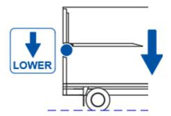
LOWER and rest the platform on the stow locks or pins, to reduce the strain on the drive system (cables, chains, pulleys, etc.) of the lift while travelling.
