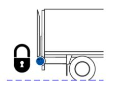
If applicable, engage the locking pins under the lift runners.
