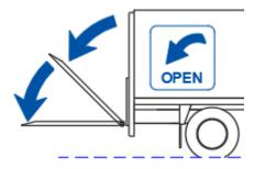
OPEN the platform into horizontal work position.
