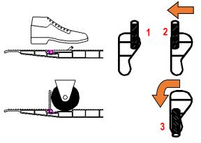
**OVP120.S.R / OVP120.A.R** = Rear or outboard retention ramps in steel or aluminium
