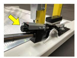
Safety valve on tilt cylinder (DH-VO)
