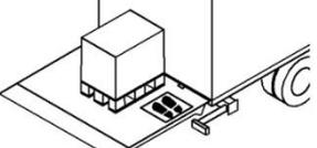
**Position load as close as possible to inboard platform edge.**
