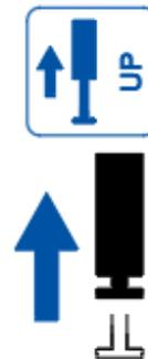
If so equipped, raise the mechanical or hydraulic stabilizing legs into travel position.
