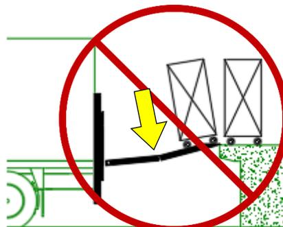
NEVER use a foldable platform as a bridge plate between the vehicle floor and a loading dock. Keep the platform securely stowed in its travel position to avoid damage.
