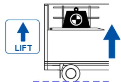
LIFT the platform, with respect for the load charts. At the highest floor, release the button when you hear the hydraulic system go in overpressure.
