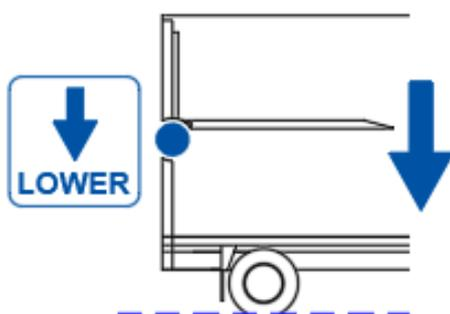
LOWER and rest the platform on the stow locks or pins, to reduce the strain on the drive system (cables, chains, pulleys, etc.) of the lift while travelling.
