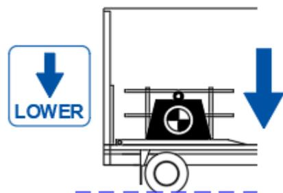
LOWER the platform to the lowest vehicle floor, with respect for the load charts.
