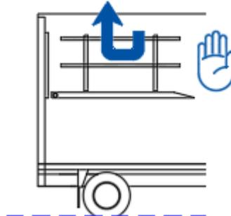
If applicable (e.g. on curtain-sider vehicle), deploy the guard rails, and lock them in vertical position.
