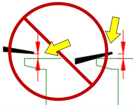
If the loading floor of the vehicle lowers or rises relative to the loading dock, use the electrical controls to adjust the platform position flush with the loading dock surface.
