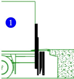
1. Platform lowered below the vehicle floor level. All cargo is loaded / unloaded over a dock-plate that links the dock and the vehicle floor.
