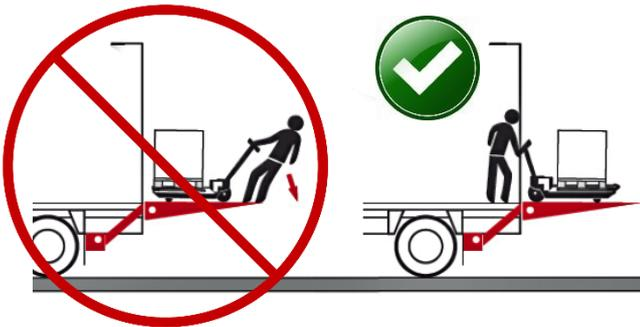
When using a second external lift to load or unload to the vehicle ground, NEVER pull the load from the vehicle onto the platform. ALWAYS push it out. Pulling the load from the vehicle can result in a fall from the platform and cause serious injury or death.
