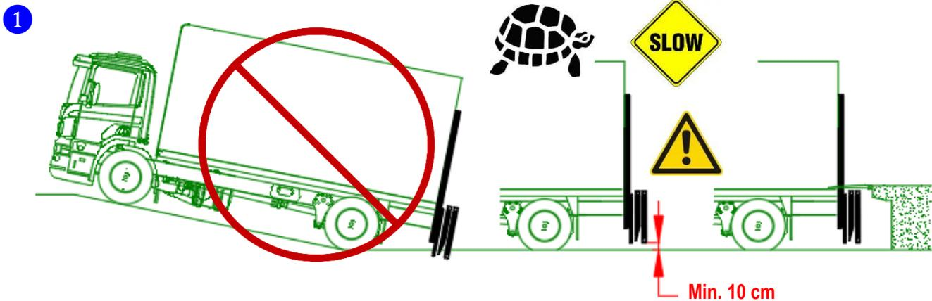
When the intention is to dock with the platform lowered below the vehicle floor level, DO NOT lower the platform until the vehicle is standing on flat even ground. ALWAYS reverse slowly, and make sure you maintain sufficient ground clearance between the lowest part of the tail lift and the ground. Take into account variations in the suspension and vehicle height.
