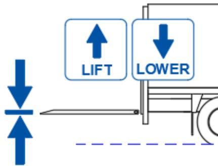
LIFT or LOWER the platform to the correct height for closing it. Normally approx. 15 cm below the vehicle floor.
