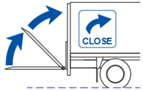
CLOSE the platform. Continue to press CLOSE until you hear the hydraulic system go in overpressure. Then release the controls.
