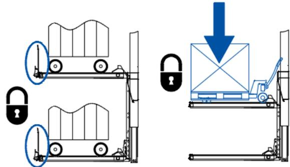
Before lifting or lowering loads, make sure the loads are secured on the platform surface. Deploy the platform cart stops (if so equipped), lower loads on a pallet jack down on the platform surface or immobilize the load via equivalent securement device.
