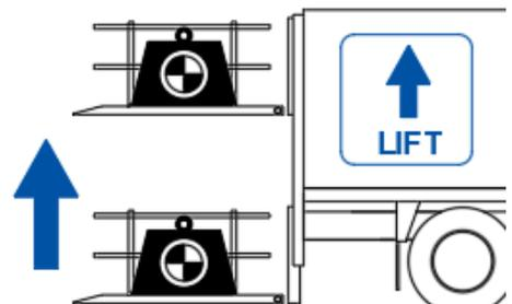
LIFT the platform off the ground, with respect for the load charts. At the highest floor, release the button when you hear the hydraulic system go in overpressure.
