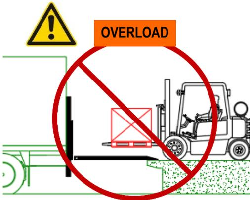
It is forbidden to drive forklifts or heavy electric pallet jacks over the platform.
