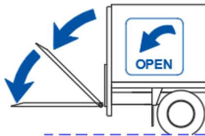
OPEN the platform into horizontal work position.
