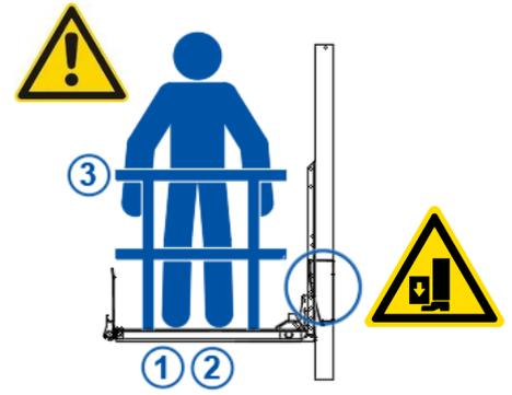
When riding on the platform, ALWAYS make sure you stand min. 250 mm away from the inboard platform edge. ALWAYS make sure your footing is solid. ALWAYS hold onto the guard rails. [see §7.5 from page 34 onwards].
