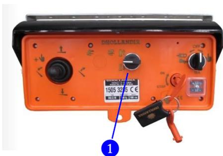
When the tail lift is equipped with hydraulic stabilizing legs, the control units above are completed by a turn switch to push the legs down or pull them up.
