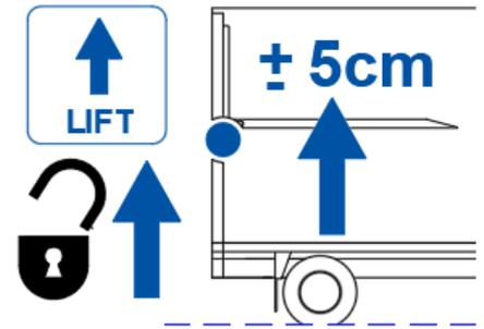
LIFT the platform approx. 5 cm to take the platform weight off the stow lock or pins.
