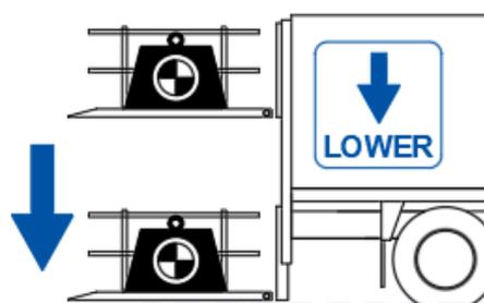
LOWER the platform to the ground, with respect for the load charts.
