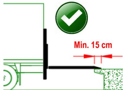
A minimum section of 15 cm of the outboard platform edge must cover the loading dock.
