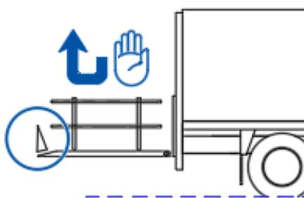
Unless unfolding automatically, deploy the guard rails and lock them in vertical position.
