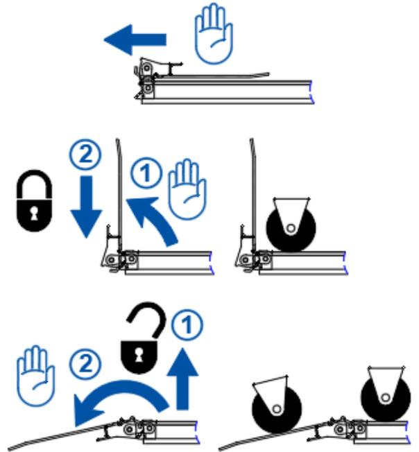
**OVP152** = Hydraulic retention ramp, electro-hydraulically operated
