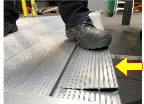
Standard toe-guard flap on exterior platform (DH-VO)
