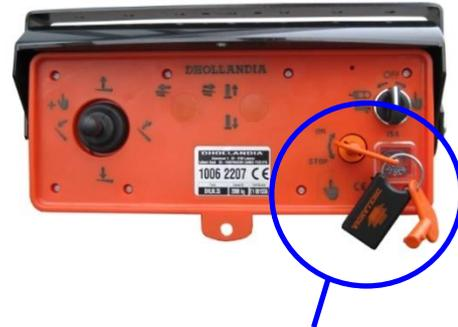
Turn clockwise to switch battery power ON
