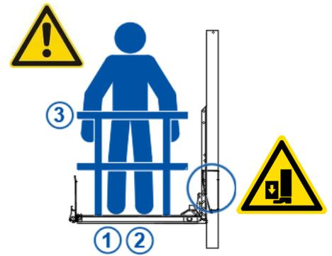
When riding on the platform, ALWAYS make sure you stand min. 25 cm away from the inboard platform edge. ALWAYS make sure your footing is solid. ALWAYS hold onto the guard rails. [see §7.5 from page 34 onwards].
