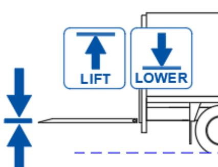
LIFT or LOWER the platform to the correct height for closing it. Normally approx. 15 cm below the vehicle floor. Use the HEIGHT DETECTION TO CLOSE for your convenience.
