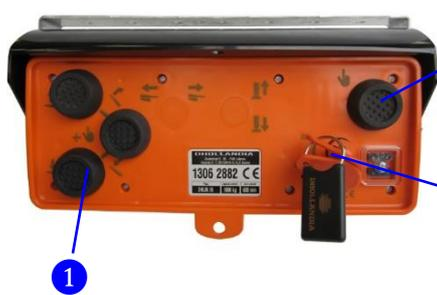
2 Push and hold to activate push buttons of main external control box
