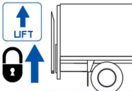
LIFT the platform until the platform stow locks are engaged. Release the button when you hear the hydraulic system go in overpressure.
