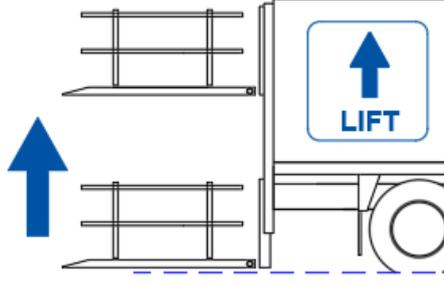
LIFT the platform off the ground. At the highest floor, continue to press LIFT until you hear the hydraulic system go in overpressure. Then, release the controls.
