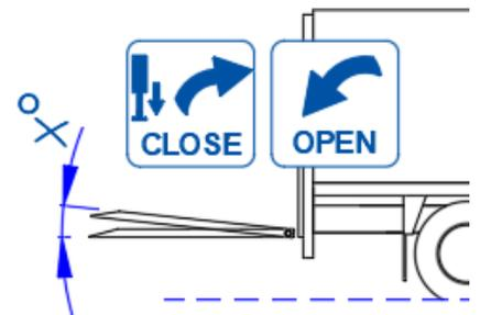
Adjust the platform pitch to compensate for the slope of the ground [see §9.1 on page 46].
