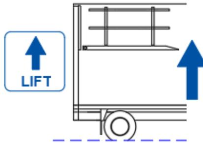
LIFT the platform. At the highest floor, release the button when you hear the hydraulic system go in overpressure.
