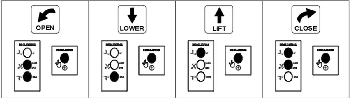
**Flush mount control unit (ref. OAE033.Z) for tail lift with hydraulic retention ramp (ref. OVP152)**
