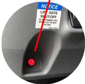
Push button to switch tail lift power ON (indicator light on)
