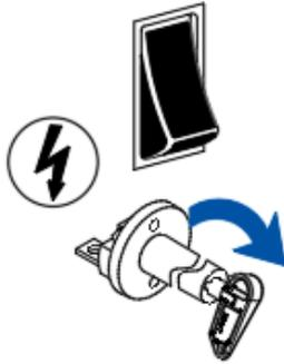
Switch on the electrical power to the tail lift (cabin switch or main battery disconnect switch in the external control box, or both if both are available).
