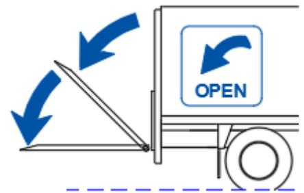
OPEN the platform into horizontal work position.
