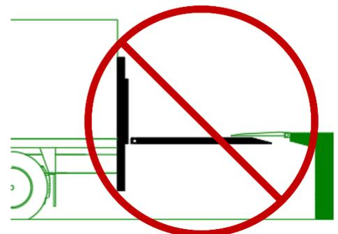
NEVER use a dock plate on top of a floating platform as a bridge between the loading dock and vehicle floor.
