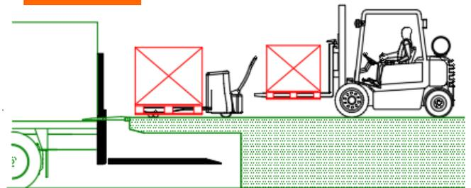
Whenever cargo is loaded or offloaded with forklifts, electric pallet jacks, and the total weight of the load plus handling equipment exceeds the maximum rated capacity of the tail lift, ALWAYS use a dock plate from the loading dock to the vehicle floor, and safely stow the lift below the vehicle floor level, or in the pocket or brief case under the loading dock.
