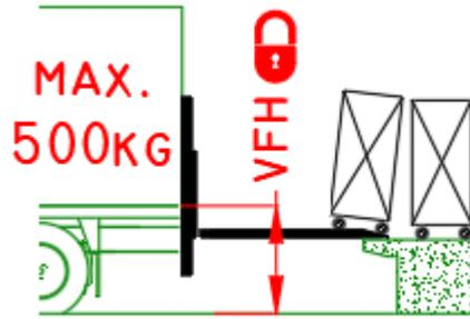
Unless the vehicle suspension can be blocked (e.g. by means of hydraulic stabilising legs) and the floor maintained at the original height vfh, the max. load transferred over the platform should not exceed 500 kg. Exception: column lifts with 2 tilt cylinders [option OVH011].
