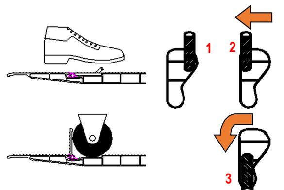
**OVP120.S.R / OVP120.A.R** = Rear or outboard retention ramps in steel or aluminium
