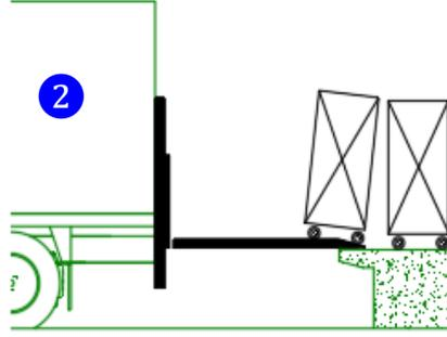
2. Platform is used as a loading platform; or as a bridge plate (in case of optional tilt cylinders)
