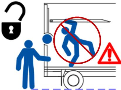
Observe all safety instructions. Disengage the stow lock or pins underneath the platform.
