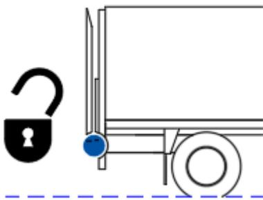
Observe all safety instructions and disengage the locking pins under the lift runners (if applicable).
