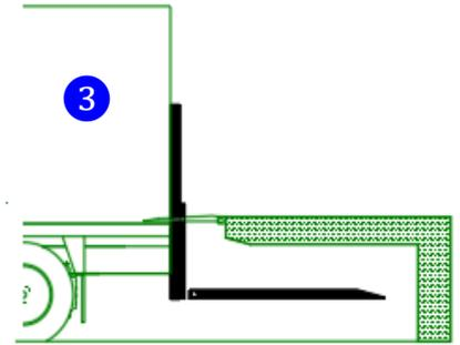
3. Platform is hidden in a pocket or briefcase under the loading dock. All cargo is loaded / unloaded over a dock-plate that links the dock and the vehicle floor.
