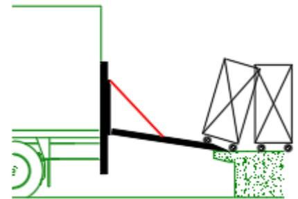
The tail lift can be used as a bridge plate, if it is equipped with the optional tilt cylinders with adjustable platform orientation [OVH011].
