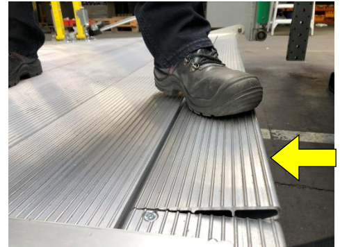
Standard toe-guard flap + toe-guard switch on exterior platform (DH-VO* / VB* / VX*)
