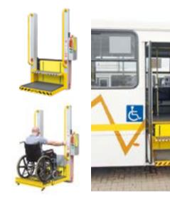
The DH-TV.03 is specially designed for **city buses**. It is mounted at the side door of the bus, and occupies the space that is otherwise occupied by the access stairs.
