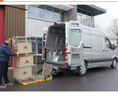
The platform of the DH-C001.03 stows neatly in a sealed cassette box under the loading floor of the vehicle. This solution keeps the access through the rear doors free, and occupies no space inside the vehicle.
