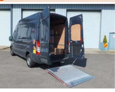
The DH-LSP.07 types 02 and 03 are derived from the basic model DH-LSP.07. Types 02 and 03 **solve a number of mounting issues** for well-defined types of vans, that couldn't be solved elegantly with the standard model.
