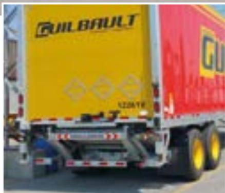
The DH-RM.25 is usually mounted underneath a reinforced bed extension plate with **2 sturdy dock-bumpers** and adjustable ladders. But it can also be mounted flush with the rear sill of the vehicle body. The fold-away storage of this lift is ideal for operations **needing frequent access to loading docks**. The optional bumper OAF105 is compatible with most common **Dock-Lock vehicle restraint systems**.
