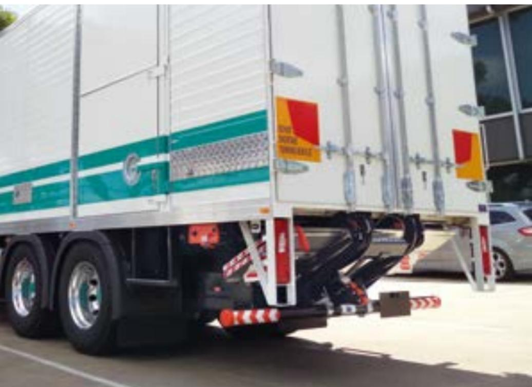
The DH-RC.15 is the medium-duty model in the range of fold-away lifts with **level ride** between the vehicle floor and the ground, plus **automatic tilt at ground level**. Despite the narrow arms situated between the chassis rails, it offers **excellent lateral stability and overall performance**.
