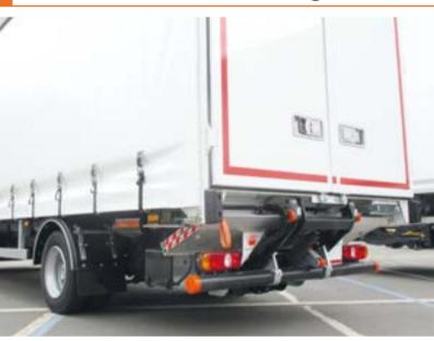
The DH-RC.10 is the light-duty alternative offering a **level ride** from the vehicle floor to the ground (and vice versa), and **automatic tilt at ground level**.
