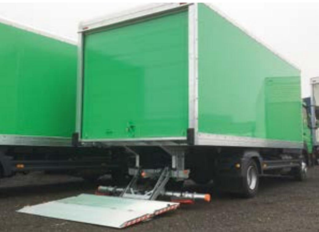
The DH-RP.10 is the middle model of 3 lifts forming a young generation of **light-weight yet robust** fold-away lifts with **half-dip platform ride** from the vehicle floor to the ground.
