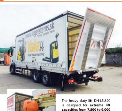
The steel platform can be extended to form the rear closure of the vehicle body and can be modified so that it can be inclined in ramp position [option OAH027].
