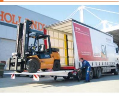
The heavy duty lift DH-LSU.60 is designed for **extreme lift capacities from 4000 to 6000 kg** and is mainly used for the transport of heavy machinery, forklifts, agricultural tractors etc...
