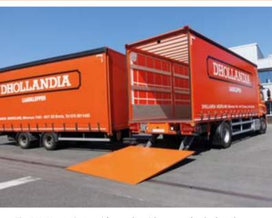
The DH-LV.40 is designed for **trucks with a central-axle draw bar trailer**, whereby the draw bar coupling is mounted deep under the truck chassis.
