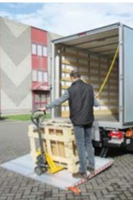
The DH-LEZ.10 is specially designed for **vertically folding platforms** [option OAP406] and offers **maximum flexibility** to the operator. When the platform stands in its travel position, one door remains free and the **driver has free access** to the cargo space inside the body. When large and heavy cargo must be handled, the platform can be opened into horizontal work position, and unfolded to a **full-width platform** in a matter of seconds.
