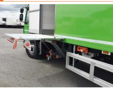
The DH-SOZ.10 replaces the fold-away lift DH-REK.10 after more than 30 years of duty, and various upgrades. It is mounted on truck chassis, in front of the rear axle, and is used to **unload or load goods at the side doors** of the truck body.
