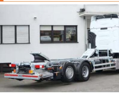
Like the other slider lifts from the DH-SO... range, the DH-SO8 is also equipped with a double folded platform, to **minimize the required installation space** behind the mud-guard or springer hangar. But this lift is mainly focused on commercial vehicles with **BDF – AWL swap bodies and containers**. Its platform consists of 3 sections: a sturdy fixed steel section, which also forms the bumper bar; and 2 light-weight aluminium folding sections.
