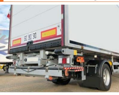
The slider lift DH-SO6 is equipped with a **double folded platform**, that rests on top of the lift arms when the lift is stowed away in its travel position, and is perfectly suited for installation on vehicles with **very short overhang** (e.g. semi-trailers with rear steering axle). Its platform is composed of 3 sections: a rugged fixed steel section, which also forms the bumper bar, and 2 light-weight folding sections.
