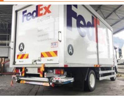
The slider lifts DH-SO... are equipped with a **double folded platform**, that rests on top of the lift arms when the lift is stowed away in its travel position. This compact construction is perfectly fit for installation on **vehicles with very short overhang**.
