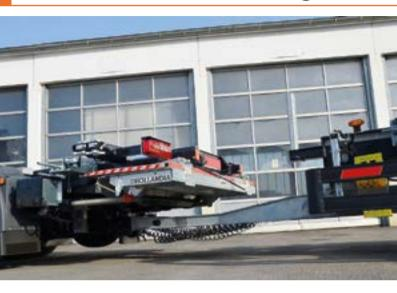
The **DH-SV** is designed for **trucks with a central-axle draw bar trailer**. In order to optimize the mounting situation, the DH-SV is **custom made** in function of the specific dimensions of the chassis, the trailer coupling and the draw bar.
