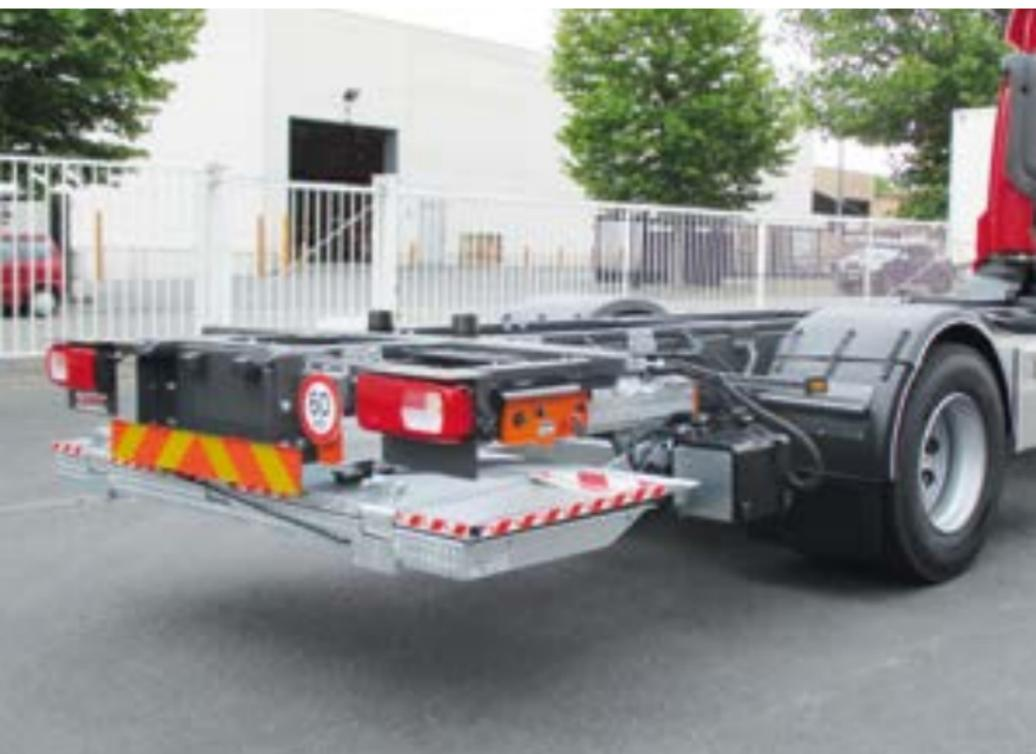
The DH-SM.15 is the **lightest of the conventional slider lifts** with single fold platforms. It is equipped with a compact lift frame and short lift arms, in order to **minimize the required overhang**. As a consequence, it is a modern and lighter weight alternative to the short overhang lift DH-SMP.20 in 1500 kg execution, and forms the ideal weight saving lift for medium capacity trucks of 7,5 T to 18 T GVW.
