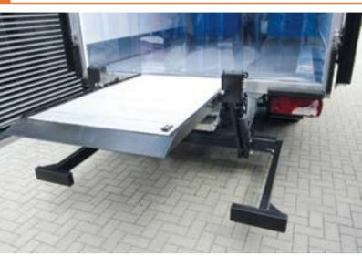
The DH-SC.05 is the **heavy-duty** version of the **CITY SLIDER lift** and is usually mounted on van chassis and light commercial trucks.
