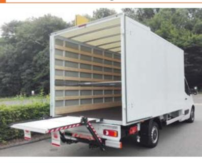
The **CITY SLIDER lift** DH-SC.04 is specially designed for mounting on van chassis and light commercial trucks.
