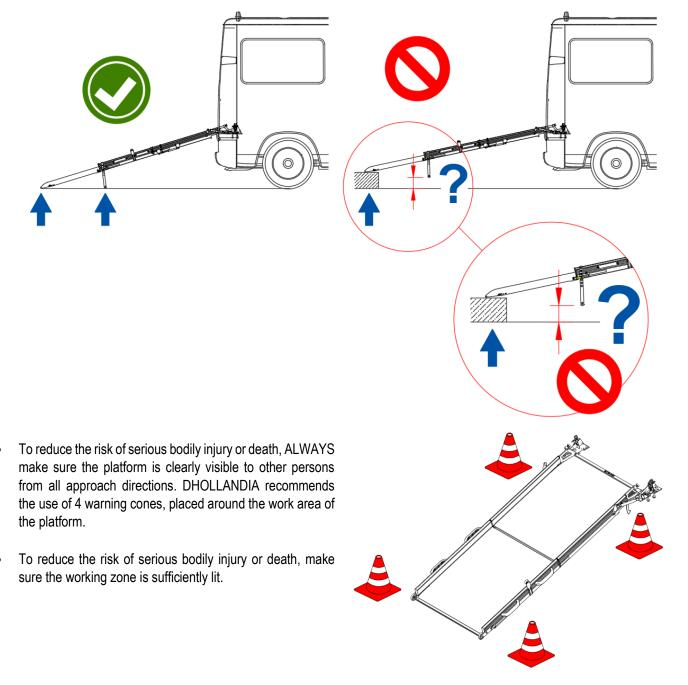
Inspect the ramp prior to each use. If any unsafe condition exists or unusual noises or movements are noticed, DO NOT use the ramp and contact an authorized DHOLLANDIA service agent for repair. Please see 'pre-trip inspection' procedures under 7.7 from page 23 onwards.
