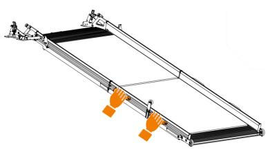
Make sure the platform is fully aligned with the ground and that the platform is supported by both wheels.
