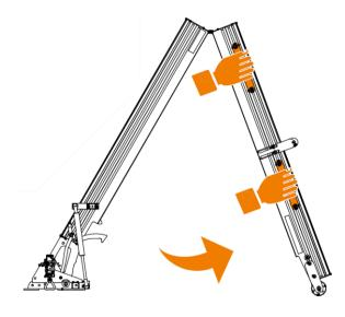
Fold open the platform and let the wheels roll on
