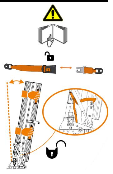
Tilt the platform. The platform lock will disengage automatically when the correct angle is reached.
