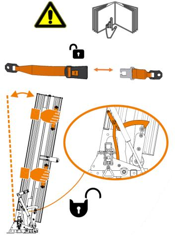
• Tilt the platform. The platform lock will disengage automatically when the correct angle is reached.
