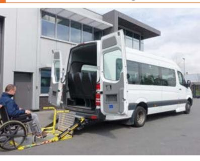
The platform of the **DH-CH001.03** stows neatly in a sealed cassette box under the chassis of a wide range of M1 - M2 minibuses. This solution keeps the **access through the rear doors free** and **occupies no space inside the vehicle**.
