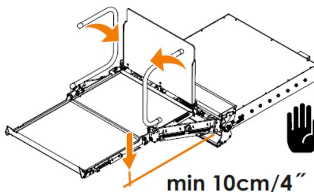
Fold the bridge plate back on top of the guard rails.
