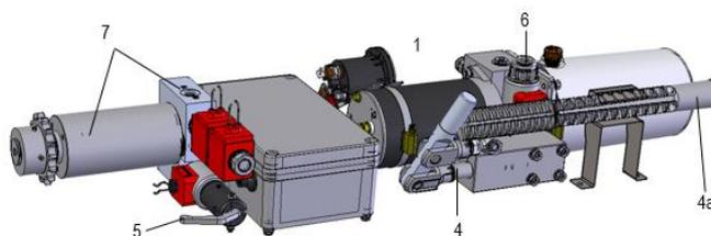
Pull the lever towards you to open that valve [5] manually.
