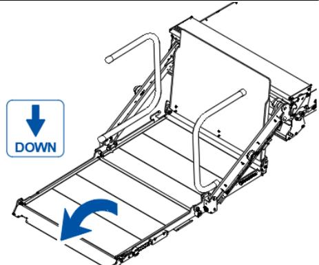
**DO NOT** step or ride off the platform before it has come to a stop at the ground, and the roll stop is fully tilted down.
