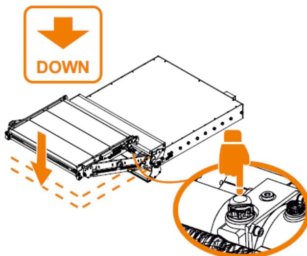
As the electrical end stop for STOW on the lift arm doesn't function in emergency mode, make sure the platform and lift arms are correctly aligned with the cassette aperture before trying to push the platform inside the cassette.
