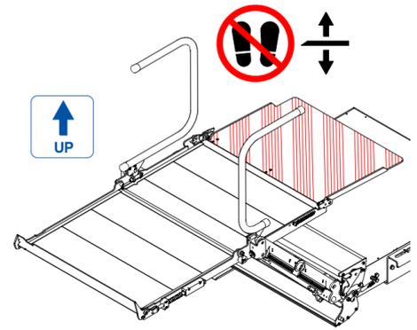
While lifting (= UP), the bridge plate will tilt down automatically as the platform approaches the vehicle floor. DO NOT stand on the bridge plate before the platform has come to a complete stop.
