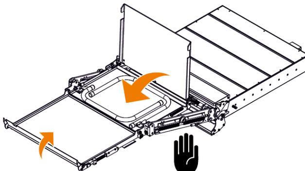
Press the Emergency Descent button [6] to lower the platform (= function LOWER) to the correct height to stow the platform.
