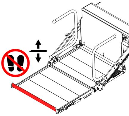
NEVER allow anybody to stand on, or hinder the roll stop at the outboard platform edge when the platform is set in motion or is in motion.
