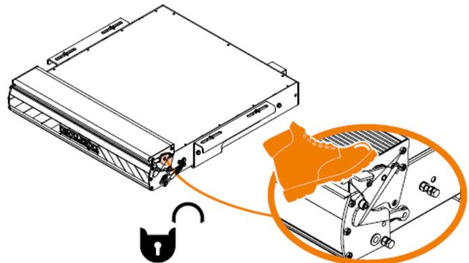
Grab the outboard edge of the folded platform and pull it out manually.
