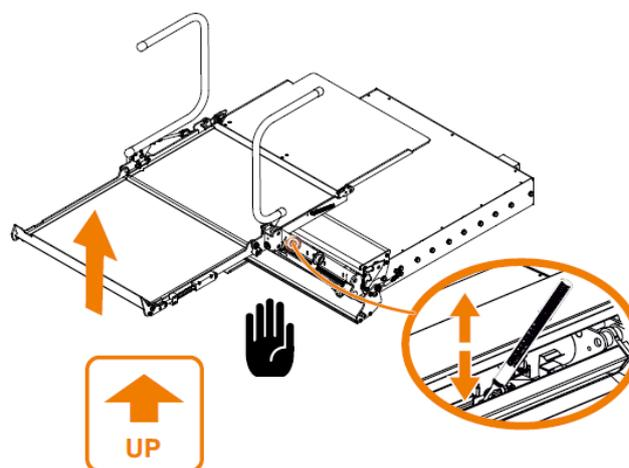
Locate the Emergency Descent button [6] on the power pack [1]. Press this button [6] continuously to lower the platform to the ground (= function LOWER) and tilt down the roll stop.
