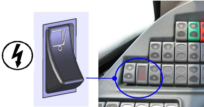
Push the button to switch the electrical power to the wheelchair lift ON.
