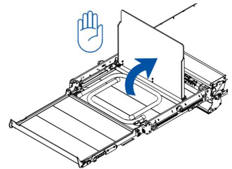
Continue to press **DEPLOY** until the platform comes to a complete stop at its dedicated work position.
