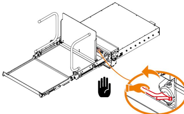
Locate the lever [4a] of the hand pump [4] at the front of the power pack [1]. Fit it over the lever arm of the hand pump.
