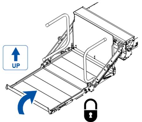
When the platform leaves the ground, **ALWAYS** make sure the roll stop is raised and secured in the upright position.
