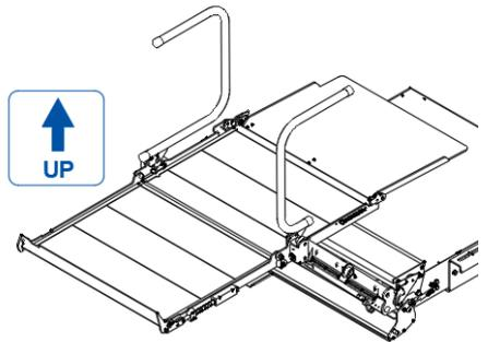
Press **UP** to raise the platform from the ground to the vehicle floor.
