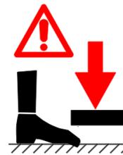
Impact by the platform or moving parts of the lift can result in bodily injury.
