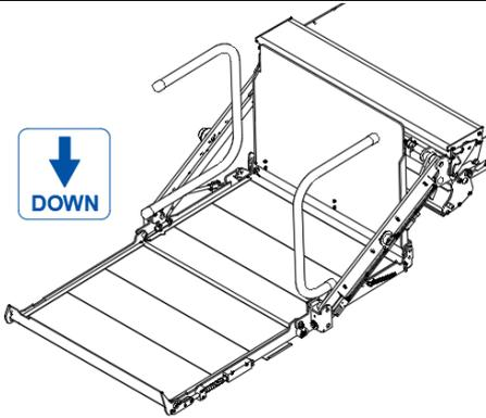
Press **DOWN** to lower the platform to the ground.
