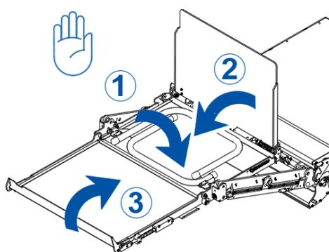
Unlock the guard rails at the left and right side of the platform. Fold back in subsequent order: the guard rails [1], then the bridge plate [2], finally the flip-over point [3].
