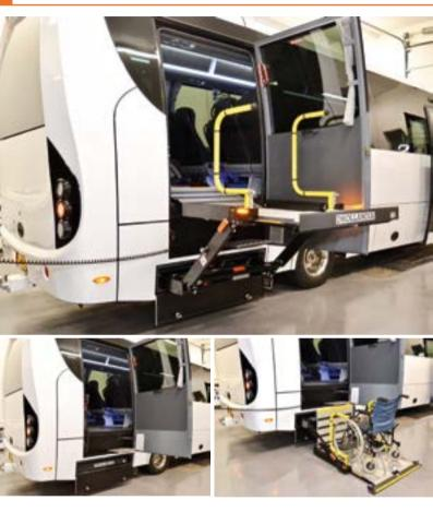
The **DH-CH003.03** is a **short cassette lift**, designed for installation at the side or at the rear door of M2-M3 buses and school buses. The lift and its platform slide in and out of the cassette by means of an electric motor. The platform is **extended manually** with **minimal effort**.
