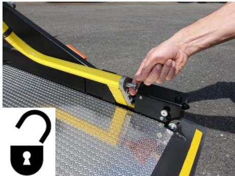
Unlock the guard rails at the left and right side of the platform.
