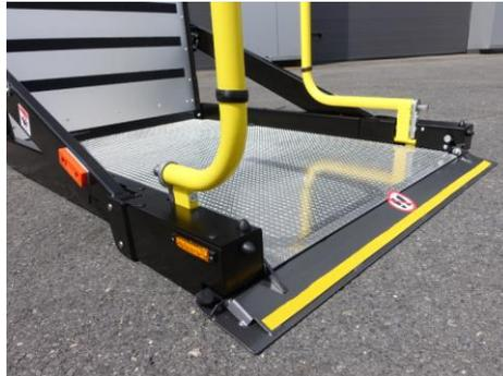
DO NOT step or ride off the platform before it has come to a stop at the ground, and the roll stop is fully tilted down.
