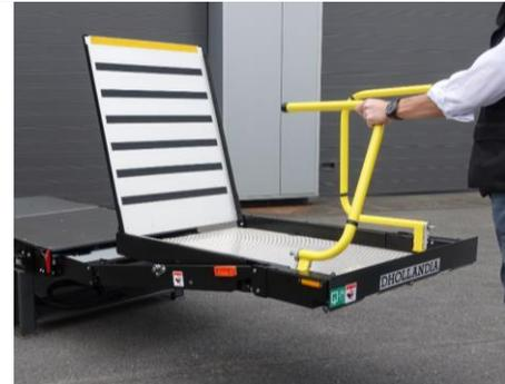
Fold the guard rails back onto the platform surface.
