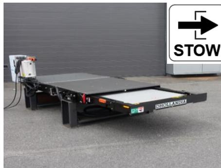
For 2-button controls, continue to press DOWN to stow the platform until it comes to a complete stop at its travel position (= STOW).
