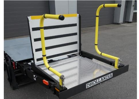
Raise the guard rails at the left and right hand side of the platform.
