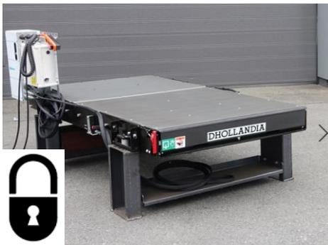
Make sure the platform is fully retracted inside the cassette and properly locked.
