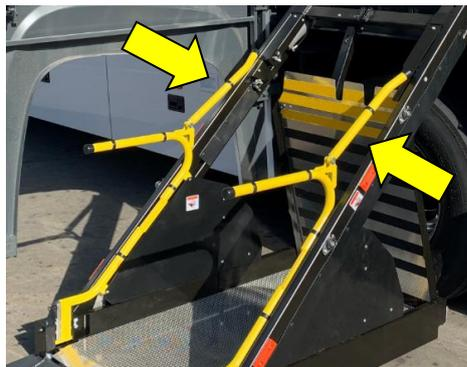
If so equipped, deploy the guard rail extensions (option OWP013).
