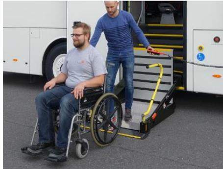
Load and unload at the ground, help wheelchair occupants embark and disembark in accordance with the instructions of section 7.4 from page 23 onwards.
