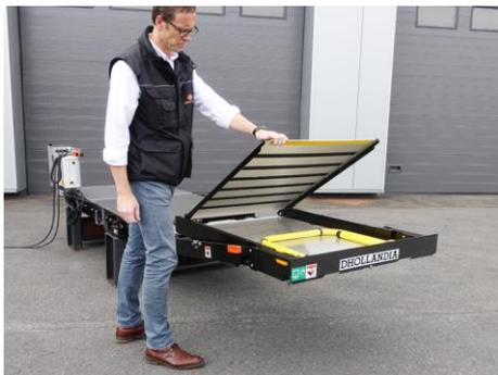
Fold the bridge plate back on top of the guard rails.
