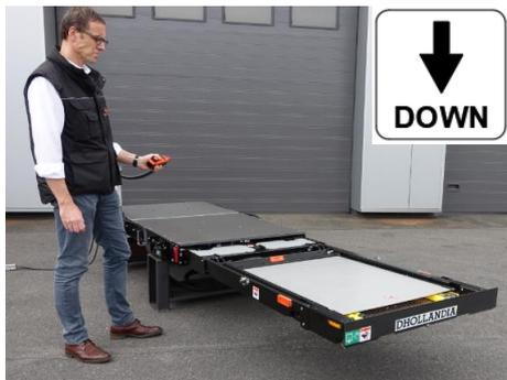
Press DOWN to lower the platform onto the end stops mounted on the lift arms.
