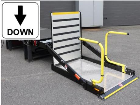
Press DOWN to lower the platform to the ground.
