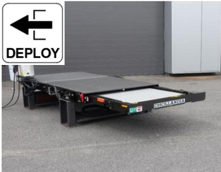
For 2-button controls, press UP to slide the platform out of the cassette.
