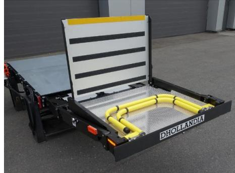
Manually open the bridge plate at the inboard platform edge.
