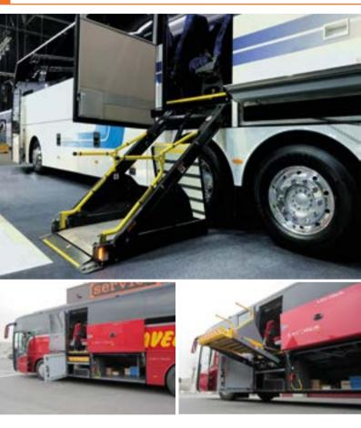
The **DH-CH101.03 and .05** are designed for installation on M3 buses and coaches, in a **compartment high above ground level**, for instance above the rear axle.
