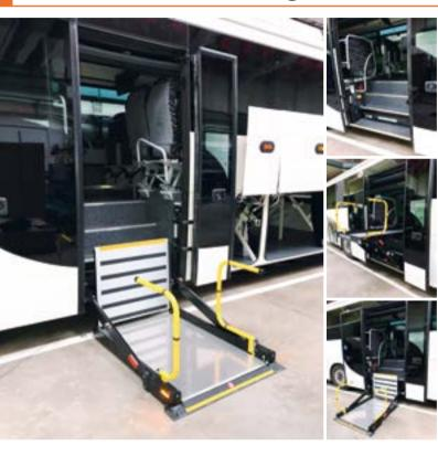
The cassette lifts **DH-CH102.03** are usually **integrated in the lowest step** of the stairs at the middle door(s) of M3 buses and coaches.
