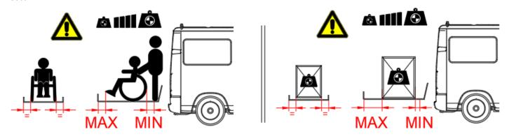
• The dimensions of the load or wheelchair should never exceed those of the platform. The load or wheelchair should never protrude beyond the perimeter of the platform.
