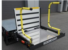
Raise the guard rails at the left and right hand side of the platform.
