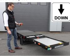
Press DOWN to lower the platform onto the end stops mounted on the lift arms.
