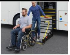
Load and unload at the ground, help wheelchair occupants embark and disembark in accordance with the instructions of section 7.4 from page 23 onwards.
