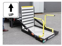
Press UP to raise the platform from the ground to the vehicle floor.
