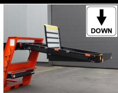
Press DOWN to lower the platform to a more convenient height, that allows the operator to raise the guard rails comfortably.
