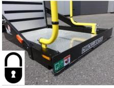
When the platform leaves the ground, ALWAYS make sure the roll stop is raised and secured in the upright position.
