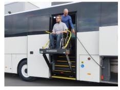
Load and unload at the vehicle floor, help wheelchair occupants embark and disembark in accordance with the instructions of section 7.4 from page 23 onwards.
