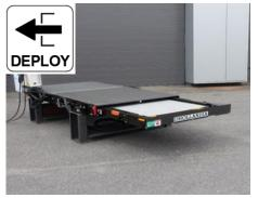
For 2-button controls, press UP to slide the platform out of the cassette. For 4-button controls, press DEPLOY to slide the platform out of the cassette. Hold the button until the platform comes to a complete stop at its dedicated work position.
