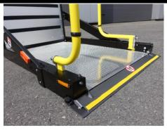
DO NOT step or ride off the platform before it has come to a stop at the ground, and the roll stop is fully tilted down.
