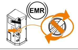
Locate the emergency cassette lock at the side of the cassette. Gently pull and release the handle to disengage the automatic cassette lock.
