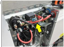
14 **Emergency descent button:** manual back-up button to lower the platform in case of an electrical power failure (= function DOWN).
