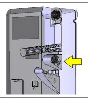
Hydraulic hand pump: manual back-up pump to lift the platform in case of an electrical power failure (= function UP).
