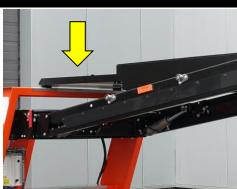
Manually open the bridge plate at the inboard platform edge.
