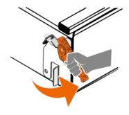
PULL the platform out by hand, until it comes to a complete stop at the dedicated work position. DO NOT apply brutal force as this may cause mechanical damage to the lift.
