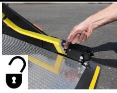
Unlock the guard rails at the left and right side of the platform.
