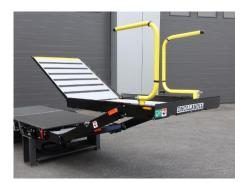
While lifting (= UP), the bridge plate will tilt down automatically as the platform approaches the vehicle floor. DO NOT stand on the bridge plate before the platform has come to a complete stop.
