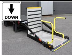
Press DOWN to lower the platform to the ground.
