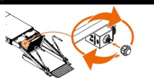
Move the lever of the hand pump up and down slowly to lift the platform (= UP). Stop at approx. 15 cm -6" above cassette height.
