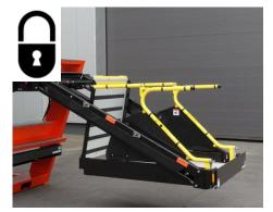
Raise the guard rails at the left and right side of the platform. ALWAYS make sure the guard rails are properly secured in the upright position.
