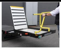
Fold the guard rails back onto the platform surface.
