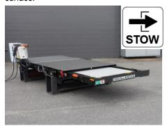
For 2-button controls, continue to press DOWN to stow the platform until it comes to a complete stop at its travel position (= STOW).
