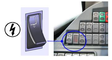
Push the button to switch the electrical power to the wheelchair lift ON
