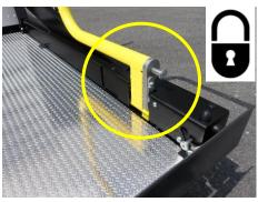
ALWAYS make sure the guard rails are properly secured in the upright position.
