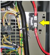
13 **15A fuse:** lighter fuses are used to protect the control unit, associated wires and the printed circuit against short circuits and amperage peaks.
