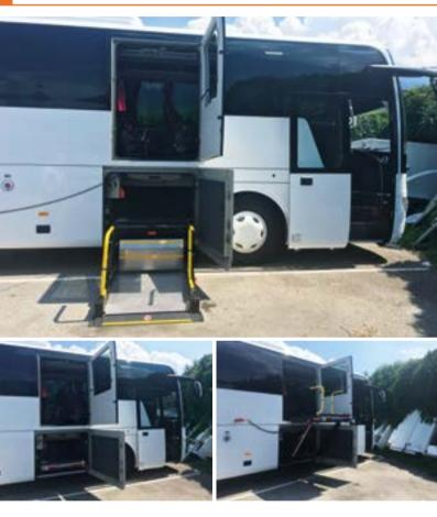
The **DH-CH103** are **heavier-duty** cassette lifts up to max. 500 kg lift capacity, usually mounted in the **luggage compartment**, or **integrated in the stairs** at the middle or front door(s) of M3 buses and coaches.
