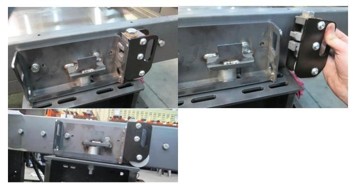
When sliding the wheelchair lift into the desired position, make sure not to damage the hydraulic and electrical connections that exit the cassette. These connections should be free and you should be able to attach them to the power pack as is explained in section 2.5.
