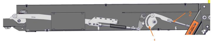
• Rod bridge plate (2): The length of the rod can be altered by releasing the counter nut and taking out the bolt that is attached to the lift arm. Turn the eye hinge to change the length of the rod. Retighten the bolt and the counter nut when finished.
