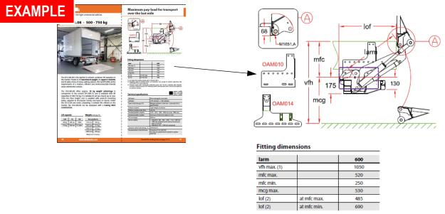
• Compare the installation dimensions and max/min installation parameters indicated in these sources with the actual vehicle dimensions. If the actual dimensions don't comply with the maximum installation parameters, DON'T continue the installation and contact your national DHOLLANDIA distributor for further advice.
