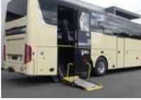
The **DH-RB.05** is a **powerful fold-away lift**, designed to embark and disembark the heaviest wheelchairs on or from coaches in a safe manner.
