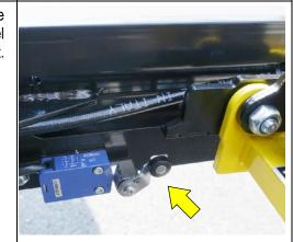
**Cabin switch** provided by the truck manufacturer or DHOLLANDIA [option OAE503.1]. This switch enables the operator to switch the control power to the lift on / off from a position in the vehicle cabin.
