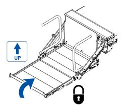
When the platform leaves the ground, ALWAYS make sure the roll stop is raised and secured in the upright position.
