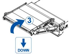
After folding the flip-over point [3] back on top of the platform main section, press DOWN to lower the platform onto the end stop mounted on the lift arm.
