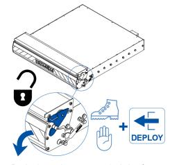
Push down the cassette lock by foot or hand and press DEPLOY to slide the platform out of the cassette.
