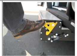
**End stop for STOW**: switch mounted on the lift arm, to automatically stop the platform at the correct height to slide in and stow the platform in its travel position. This system prevents trial and error, and mechanical damage of the lift.
