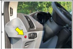
**Main battery fuse:** a main fuse 100 – 150A is supplied by the vehicle manufacturer or by DHOLLANDIA. It protects the main battery cable from the batteries to the power pack of the lift against short circuits and amperage peaks.
