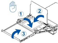
Unlock the guard rails at the left and right side of the platform. Fold back on subsequent order: the guard rails [1], then the bridge plate [2], finally the flip-over point [3].
