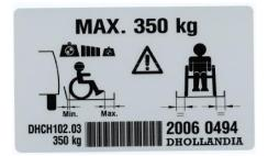
Medium sized labels are affixed to the lift frame, to the platform and to the power pack.
