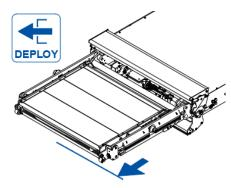
Continue to press DEPLOY until the Manually unfold the flip-over point. platform comes to a complete stop at its dedicated work position.
