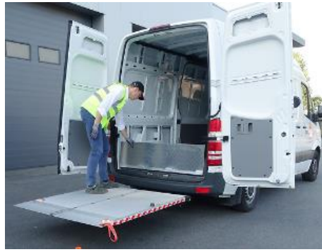
Manually deploy the bridge plate.
