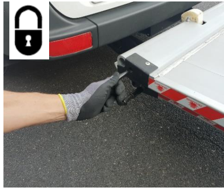
Engage the platform fold lock firmly.
