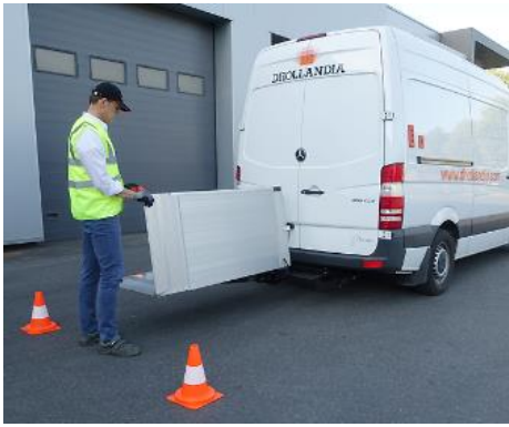
Fold the flip-over point back on the platform main section.
