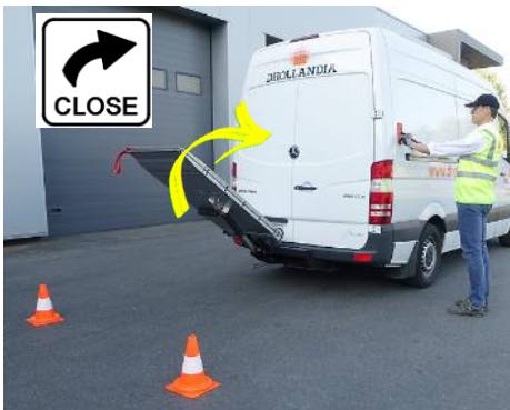
CLOSE the platform until it reaches the closed vertical position and you hear the hydraulic system turn in overpressure.
