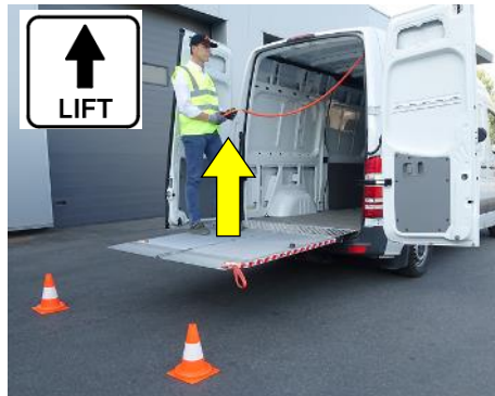
LIFT the platform off the ground. Use the AUTOMATIC TILT to return the platform to level orientation. If riding on the platform, DON'T place your feet beyond the inboard platform edge.
