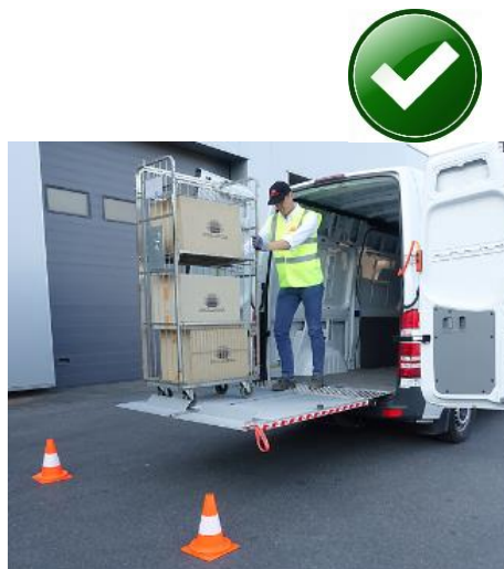
NEVER pull the load from the vehicle onto the platform. ALWAYS push it out. Pulling the load from the vehicle can result in a fall from the platform and cause serious injury or death.
