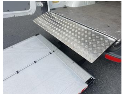
When LIFTED fully, the platform will line up with the bridge plate and connect to the vehicle floor. Release the buttons when you hear the hydraulic system turn in overpressure.
