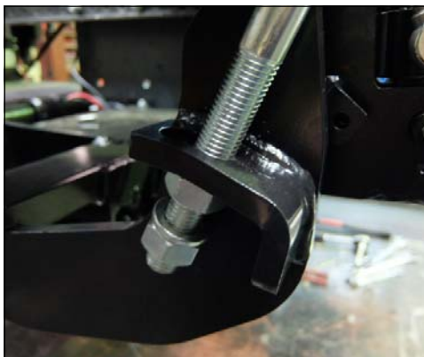
Tighten 1st nut of tension rod: 1. turn nut CW until it hits the steel holder 2. Use key to turn nut further 1 full turn of 360°
