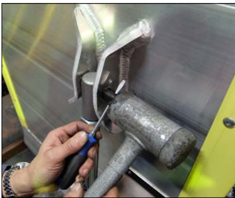
Mount articulation pin back through mounting plates on platform and through tilt cylinder extension.
