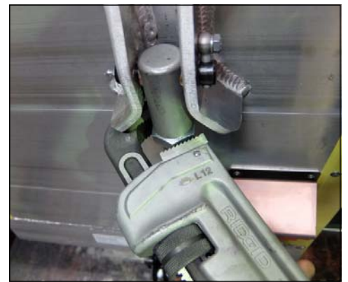
Fasten counter-nut tight against underside of tilt cylinder extension rod.
