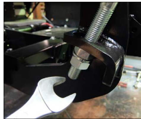
Insert spring washer between the 2 nuts. Use key to fasten counter-nut tight against 1st nut. Fast nut with required torque.
