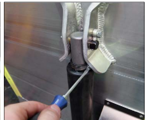
Bring rubber gaiter back in correct position, and tighten collar.
