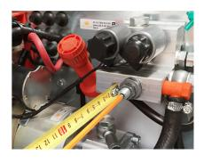
While unscrewing the center pressure screw, measure and make sure you always keep the bottom end min. 4 mm or 5/32" inside the base of the cartridge. Press LIFT for 30 sec.
