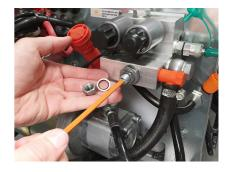
This procedure will require that you unscrew the center pressure screw while the pump is running and building up pressure.
