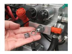
Remove the cap of the pressure relief valve, loosen the jam nut (CCW).
