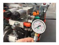
Attach a pressure gauge K0106 (or equivalent) on the pressure gauge coupling
