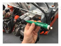
Test of solenoid on control valve in pump unit
