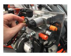
Manual operation of single acting control valve H (LIFT) in pump unit
