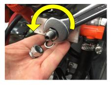
Remove the cap of the pressure relief valve, loosen the jam nut (CCW).
