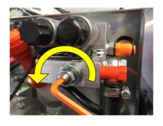
Press LIFT to make the pump run.
