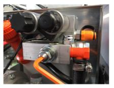
Turn CCW = lower pressure and lift capacity
