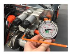
Increase the load on the platform by 10%. Adjust the pressure so that the tail lift can NOT lift the max. rated capacity + 10%.
