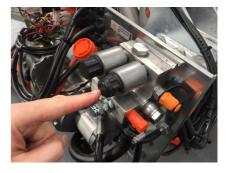
Manual operation of double acting control valve S (OPEN - CLOSE) in pump unit
