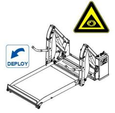
Check if the guard rails [W] are deployed in their active position.
