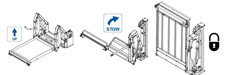
Press UP to raise the platform to the vehicle floor.
