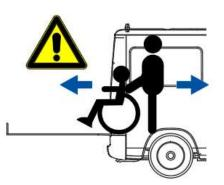
Load and unload at the vehicle floor, help wheelchair occupants embark and disembark in accordance with the instructions of section 7.4 from page 22 onwards.
