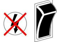
Switch OFF the electrical power to the lift by means of the cabin switch and / or the main battery disconnect switch on the power pack.
