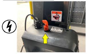
Turn the key clockwise to switch the battery power ON. Turn the key counter-clockwise to switch the battery power OFF.
