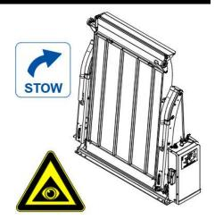
Press STOW. Check if the hydraulic system is building up pressure and the platform is pressing hard against the lift arms.
