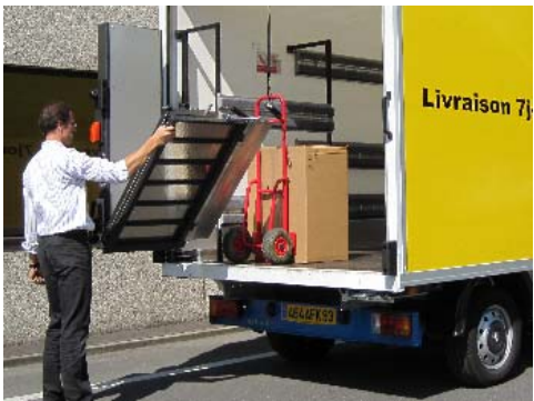
Open the platform from the vertical stow position to the horizontal work position
