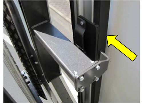
Verify if the upper support hook is properly engaged in the corresponding bracket on the side of the vehicle body
