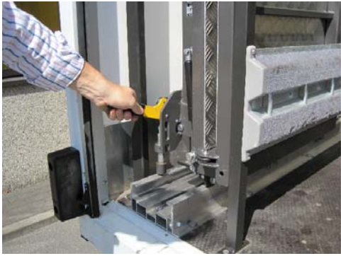
Release the mechanical travel lock
