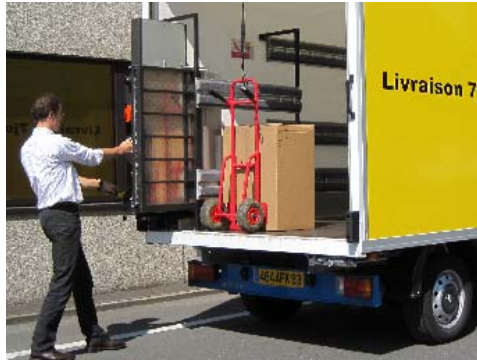
Grab the plastic handle on the lift frame, and pull the frame back until it hits the end of the sliding tube
