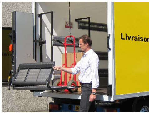
Unfold the platform point. Beware of hand and finger traps.
