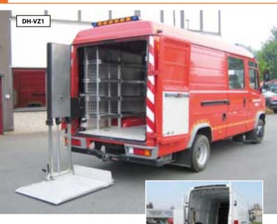
The interior column lift DH-VZ is designed to suit a wide range of Multi Passenger Vehicles, vans, and even larger commercial vehicles.
