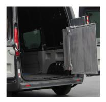
Position behind the vehicle. Now unfold the platform. Beware of hand and finger traps.
