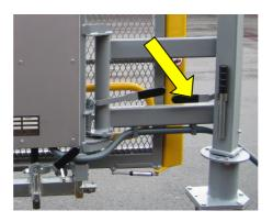
Release the rotation lock and manually rotate the lift 90° or 180° until the lift is behind the vehicle.
