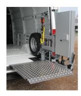
Release the rotation lock of the lift body and manually rotate the lift body back to is resting on the loading floor. the position behind the vehicle.
