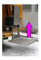
Use to controls to LIFT the platform to the loading floor level of the vehicle. Release the LIFT button when the platform has reached its highest position
