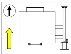
Press LIFT to check if the hydraulic system is building up pressure, and there is no visual oil leaks.
