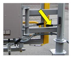
Release the rotation lock and manually rotate the lift  $90^{\circ}$  or  $180^{\circ}$  until the lift is in stored position.
