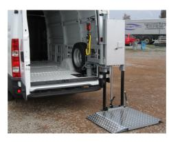
Do not load / offload the platform before it has reached its final parking position at the ground
