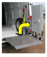
Fold the platform back into vertical position. Beware of hand and finger traps.
