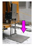
Lower the platform to the ground (or pavement at the roadside)
