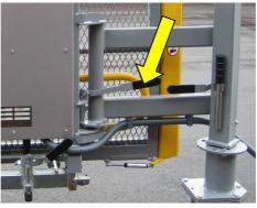
Release the second rotation lock in order to rotate the lift body.
