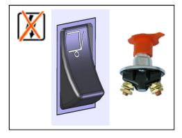
Switch off the electrical power to the lift (cabin switch in the driver's cabin, or main battery isolator switch)
