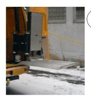
Rotate the lift 90° outwards to bring it in the position where it can start lowering
