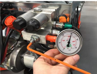
Use an Allen key or screwdriver to adjust the center pressure screw. Press LIFT. Adjust the pressure screw so the platform just lifts the max. rated capacity.
