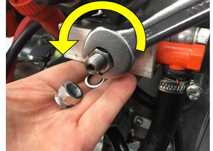
Remove the cap of the pressure relief valve, loosen the jam nut (CCW).
