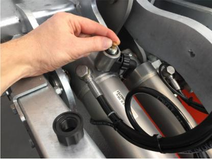
Manual operation of single acting cylinder lock valve O (OPEN) or D (DOWN)
