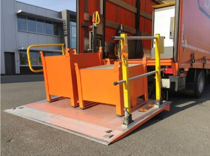
Place a load corresponding with the max. rated capacity at the correct center point of max. load on the platform.
