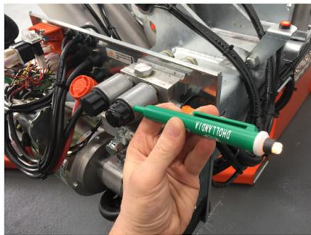
Test of solenoid on control valve in pump unit
