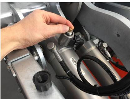
Manual operation of single acting cylinder lock valve O (OPEN) or D (DOWN)
