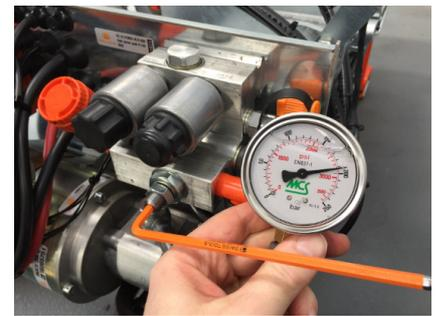
Increase the load on the platform by 10%. Adjust the pressure so that the tail lift can NOT lift the max. rated capacity + 10%.
