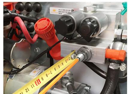
While unscrewing the center pressure screw, measure and make sure you always keep the bottom end min. 4 mm or 5/32" inside the base of the cartridge. Press LIFT for 30 sec.
