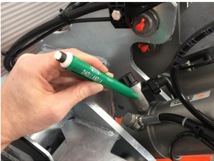
Test of solenoid on cylinder lock valve
