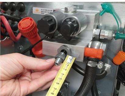
Rest the platform at the ground to dump all hydraulic pressure in the system.
