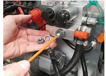
This procedure will require that you unscrew the center pressure screw while the pump is running and building up pressure.
