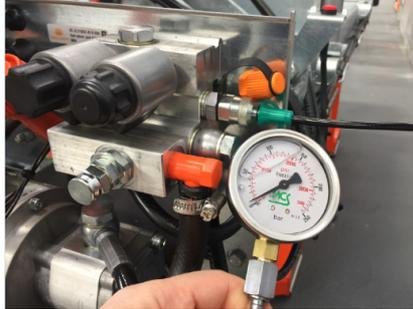
Attach a pressure gauge K0106 (or equivalent) on the pressure gauge coupling
