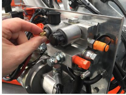
Manual operation of single acting control valve H (LIFT) in pump unit
