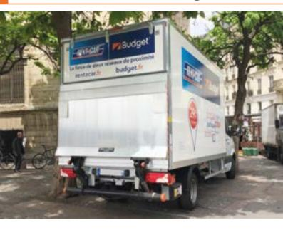
The DH-LE is a **light-weight 2-cylinder lift**, at the entry level of DHOLLANDIA's range of cantilever lifts. Thanks to its compact lift frame and short lift arms, it ideally suits light commercial vehicles with **very short overhang**.
