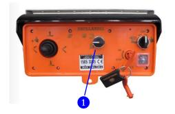
When the tail lift is equipped with hydraulic stabilizing legs, the control units above are completed by a turn switch to push the legs down or pull them up.
