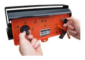
• Tail lift on/off switch [min. 1 compulsory]. Depending on configuration, the electrical power to the tail lift is switched on / off by
