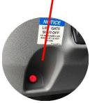
Push button to switch tail lift power ON (indicator light on)
