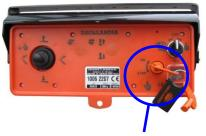
Turn clockwise to switch battery power ON
