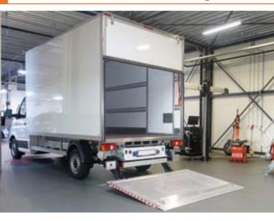
The DH-LMA.08 is the lightest 4-cylinder cantilever lift available on the market. Thanks to its **benchmark weight**, its **superior stability** and its wide choice of value-adding options, this tail lift fulfills all the requirements of a modern, efficient and environmentally friendly urban distribution vehicle.
